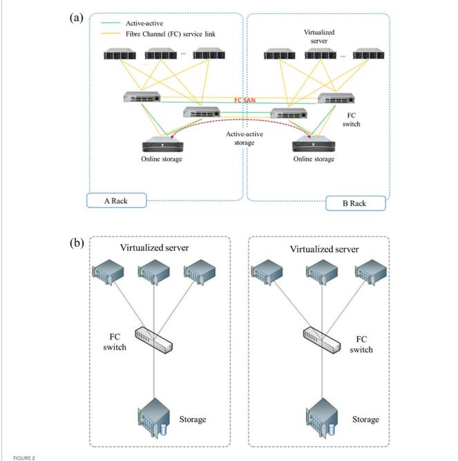
Redundant network architecture: (a) Dual-Active Architecture with a direct link for state mirroring and the dual-active manager facilitating automatic failover; (b) Independent Operation Architecture, showing two separate virtualization clusters with distributed monitoring nodes and routed network connectivity between them.
