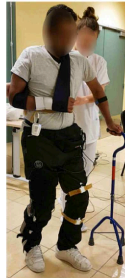
FIGURE 6 | Architecture used for knee control. Subject equipped with inertial measurement unit sensors, stimulator and controller (© Inria / Photo L. Jacq).
