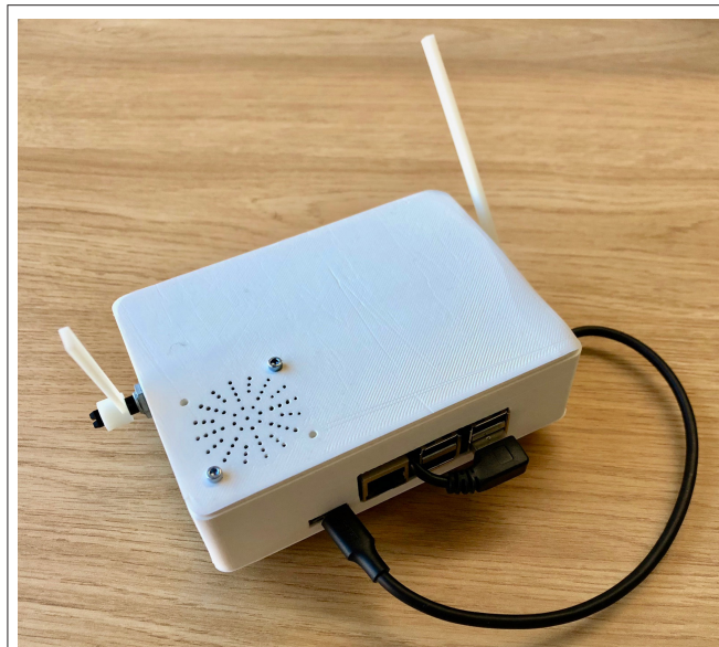
FIGURE 1 | The Embodied Music Prediction Interface (EMPI) prototype. The system includes a lever for a performer's physical input (left side) and a motor-controlled lever for physical output, a speaker, and Raspberry Pi. This system represents a minimum set of inputs and outputs to experiment with embodied predictive interaction. A demonstration video can be viewed in the Supplementary Material .
