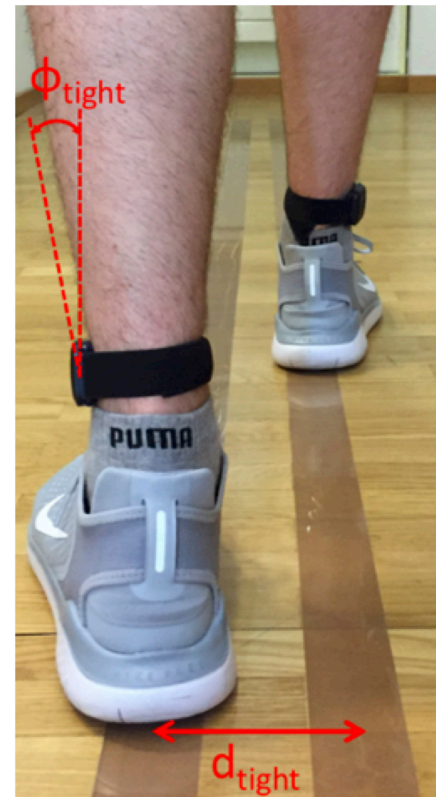
FIGURE 3 | Principle of step width (SW) calibration procedure. The subject walked on two parallel lines, spaced by d_{tight} or d_{broad} , for which the tilting angles \Phi_{tight} and \Phi_{broad} were evaluated. These four values were used to define a linear reference line for the SW estimation where the \Phi values were matched to d values between the feet.
