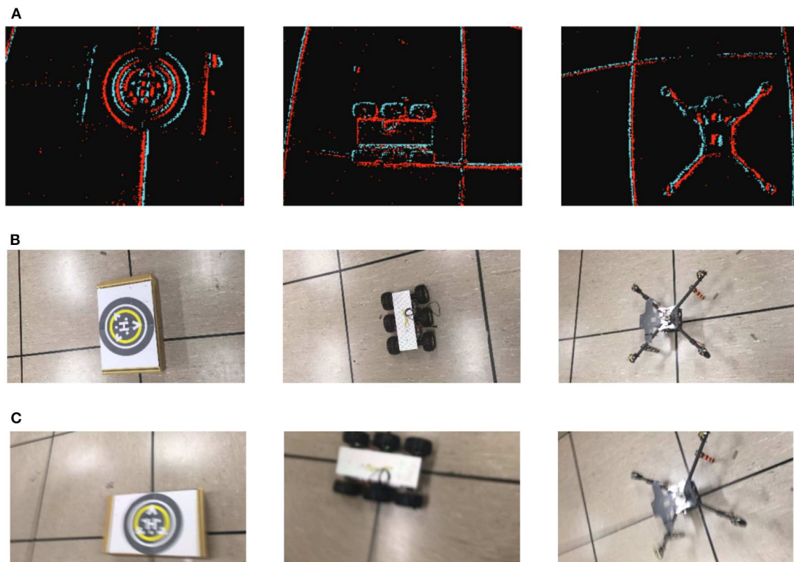
FIGURE 5 | Samples from the in-house datasets containing a Landing platform, UAV and Thumper (Empty Floor as background class): (A) N-SOD dataset, (B) Frame-based dataset similar to N-SOD, (C) Frame-based dataset with blur similar to N-SOD.
