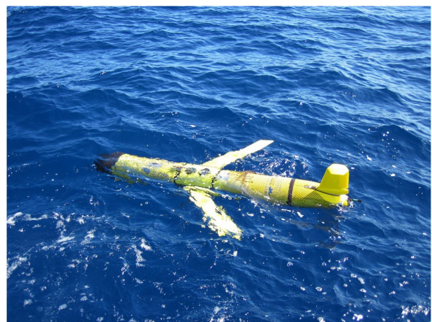
FIGURE 5 | Slocum glider during DP02 cruise deployment.
