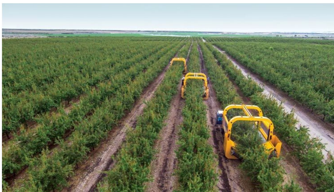
FIGURE 4 | Catch-frame harvesting of almonds in Spain using specialized equipment integrating tree-shakers and collection frames for catching harvested fruit (hulls plus nuts) before they hit the ground.
