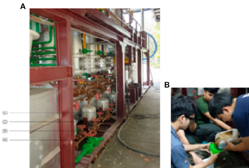
FIGURE 4 | Collecting pyrolysis oil samples (A) four collecting areas and (B) Collecting the condensed pyrolysis oil.
