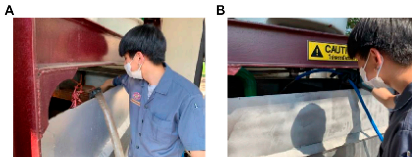
FIGURE 2 | Preparation of the coolant (A) Taking remain water out of the coolant tank and (B) Adding new water into the tank.
