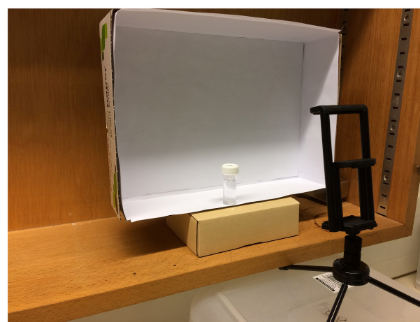
FIGURE 1 | Set up showing the sample and tripod positioning for photographic chlorophyll analysis.
