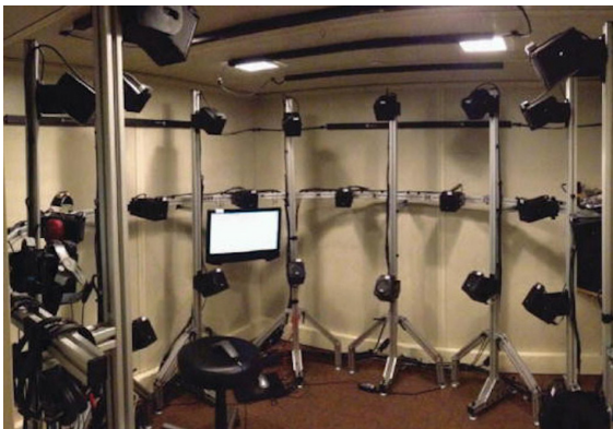
FIGURE 2 | Example of a loudspeaker array used to test localization ability by identification of the loudspeaker from which a test signal has been presented. Such arrays can also be used to test spatial release from masking with speech or other stimuli. See text for experimental details. Reproduced with permission from Brungart et al. (2017). Copyright 2017, Acoustical Society of America.
