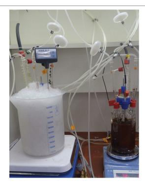
**FIGURE 1** | Cultures of *M. sedula* at cold temperature regime. Fermentation set up for cultivation of *M. sedula* in 1L glassblower modified Schott-bottle bioreactors at 73°C (right) and at cold temperature regime in ice-supplemented environment with a tap water heat exchange system (left).
