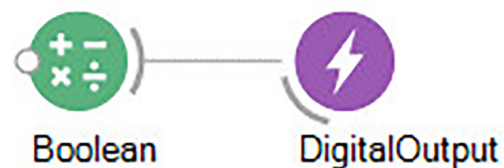
FIGURE 8 | Bonsai workflow for controlling a single Arduino digital output.
