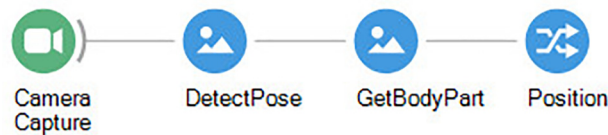
FIGURE 6 | Bonsai workflow for tracking a specific body part using the Bonsai-DLC package.
