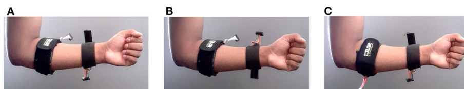
FIGURE 13 | Three placements of sensor bands, (A) two FSR1 from SB_e and SB_w are aligned with brachioradialis and near insertion of brachioradialis, (B) aligned with brachioradialis and flexor carpi ulnaris, (C) aligned with palmaris longus and near insertion of brachioradialis.
