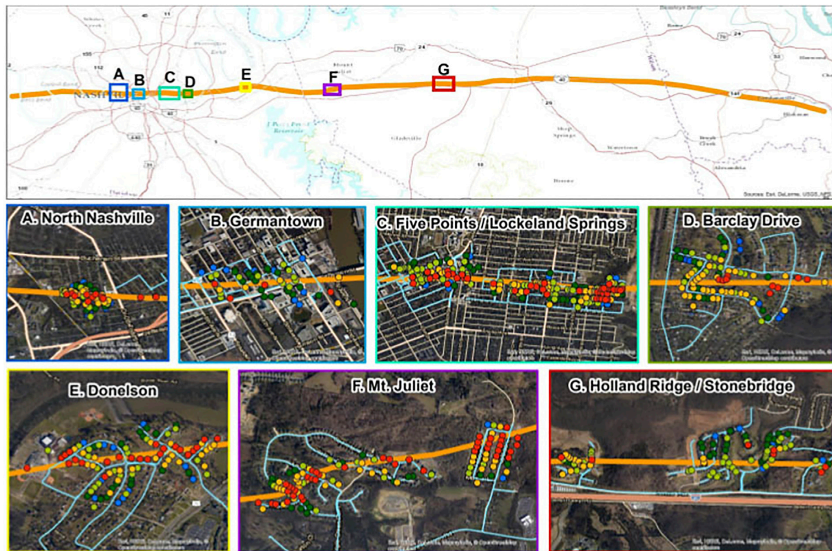
FIGURE 5 | StEER FAST app-based structural assessments in response to the Nashville tornadoes in key geographic regions relative to the tornado centerline. Blue lines in the detail plots indicate routes captured with street-level panoramas. Colored circles indicate locations of app-based structural assessments, where red to blue shading indicates high to low severity of damage.
