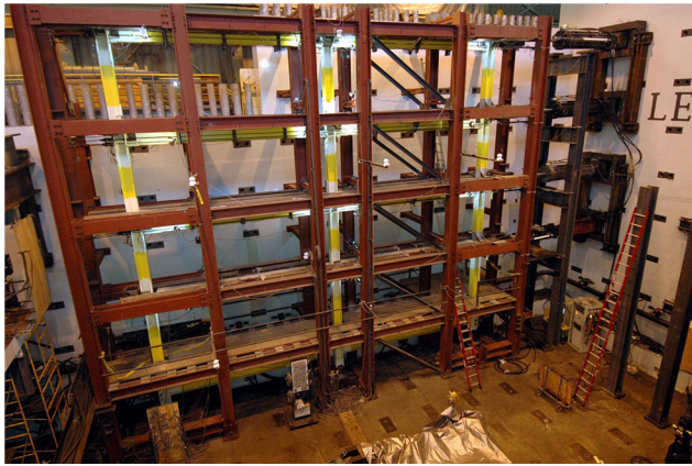
FIGURE 2 | Large-scale hybrid simulation of a self-centering steel moment-resisting frame building under simulated earthquake loading. (Photo: Jim Ricies).
