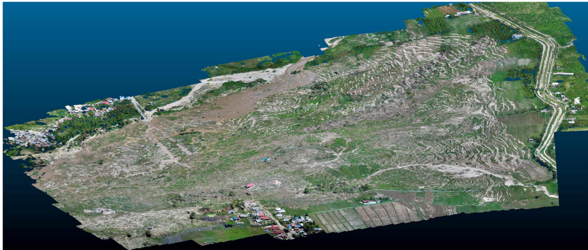
FIGURE 10 | True-color digital surface model (shown as a “point cloud”) of a flowslide.
