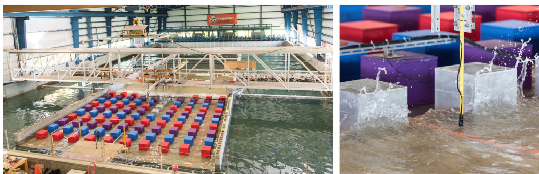
FIGURE 13 | Setup of overland flow in DWB ( left ) and detail of wave impact on coastal structures ( right ).
