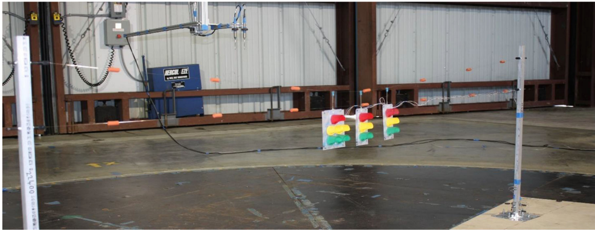
FIGURE 4 | Aeroelastic model on the WOW turntable.
