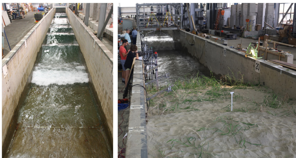
FIGURE 2 | Large Wave Flume overview ( left ) and use of LWF for dune erosion study ( right ).
