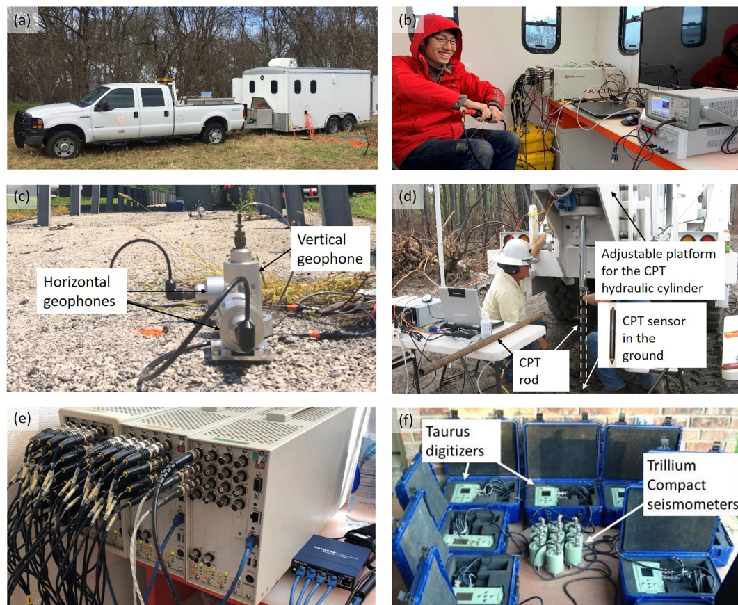
FIGURE 3 | Photographs of the field supply truck, mobile instrumentation trailer and some associated instrumentation available at NHERI@UTexas: (a) Field supply truck and instrumentation trailer, (b) Air-conditioned work space in instrumentation trailer, (c) 1-Hz vertical geophones and cables, (d) Cone penetrometer test equipment, (e) Data Physics analyzers, and (f) Trillium Compact Seismometers and Taurus Digitizers (after Stokoe et al., 2017).
