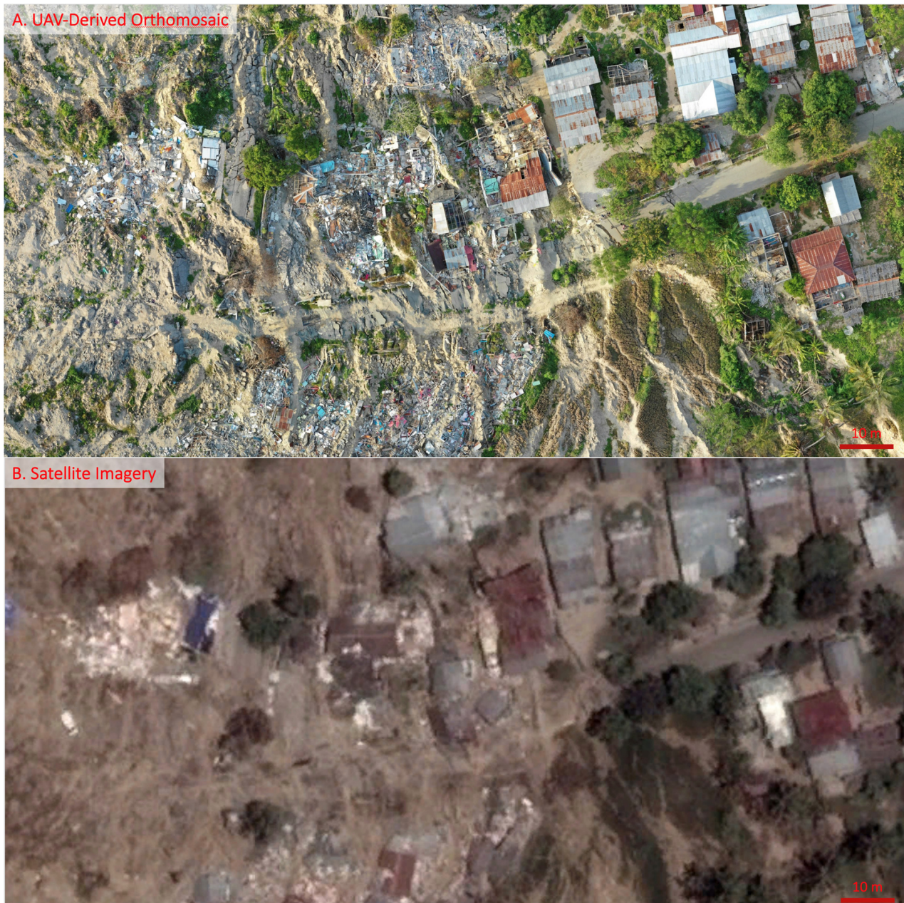
FIGURE 9 | (A) Example of a portion of a high-resolution ( \sim 2 cm pixel) orthomosaic of a flowslide. (B) Shown for comparison is a post-earthquake satellite image of the same scene provided by Google Earth crisis response program. Note the dramatic difference in resolution between the images.
