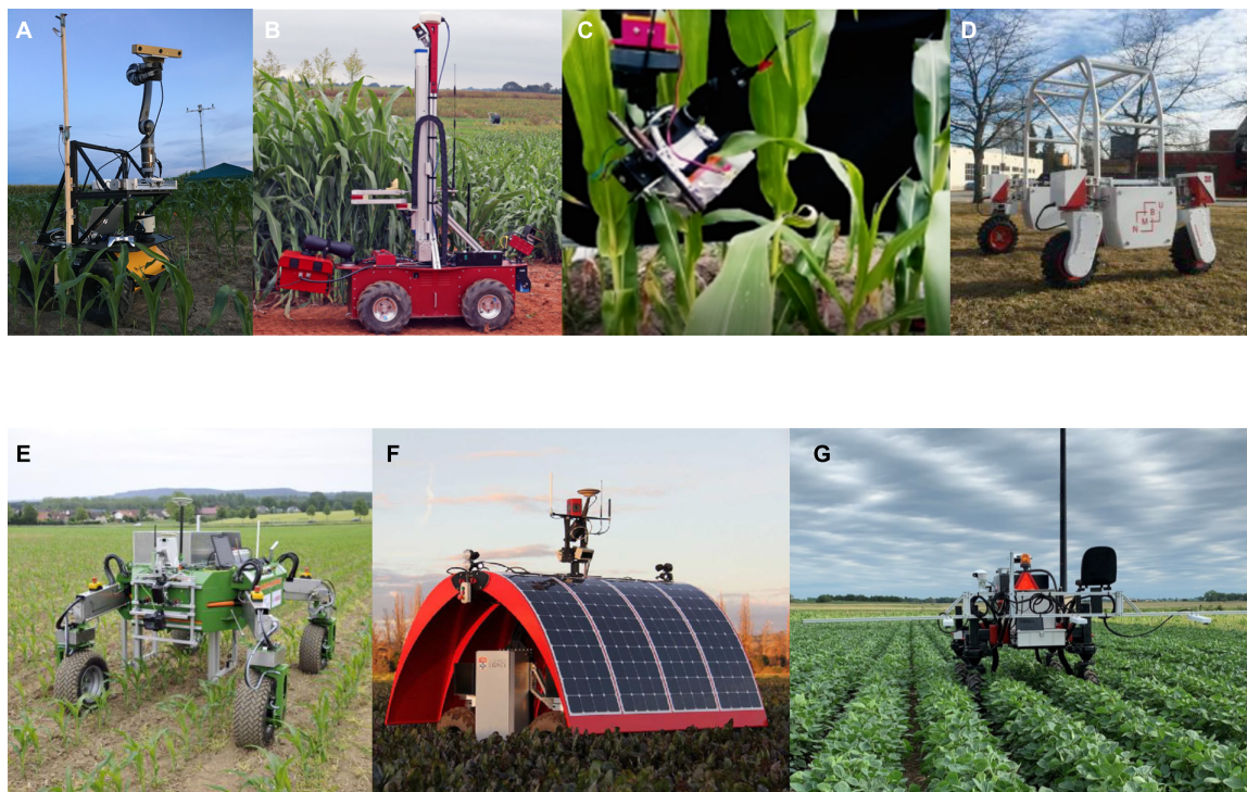
FIGURE 3 | Plant phenotyping systems for outdoor environment: (A) Vinobot: robotic system including six DOF robotic manipulator and a 3D imaging sensor mounting on a mobile platform to measure plant height and LAI (Shafiekhani et al., 2017), (B) Robotanist: UGV-based robotic system equipped with a three DOF robotic manipulator and a force gauge for stalk strength measurement (Mueller-Sim et al., 2017), (C) A robotic system to slide LeafSpec across entire leaf to collect its hyperspectral images (Chen et al., 2021), (D) Thorvald II: VIS/NIR multispectral camera mounted on a mobile robot to measure NDVI (Grimstad and From, 2017), (E) BoniRob: autonomous robot platform using spectral imaging and 3D TOF cameras to measure plant height, stem thickness, biomass, and spectral reflection (Biber et al., 2012), (F) Ladybird: ground-based system consisted of a hyperspectral camera, a stereo camera, a thermal camera, and LIDAR to measure crop height, crop closure, and NDVI (Underwood et al., 2017), and (G) Flex-Ro: high-throughput plant phenotyping system equipped with a passive fiber optic, a RGB camera, an ultrasonic distance sensor, and an infrared radiometer for the measurement of NDVI, canopy coverage, and canopy height (Murman, 2019).
