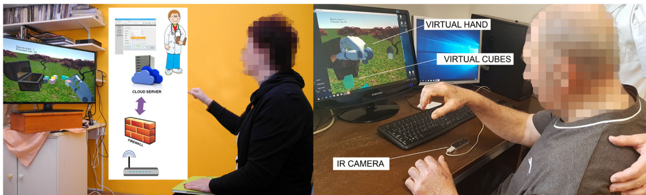
FIGURE 2 | Participants at exergaming in home (left) and hospital (right) environment. Both groups used the same 10Cubes game and LMC. The telerehabilitation system for the home group recorded the data locally and transferred afterwards to the server.
