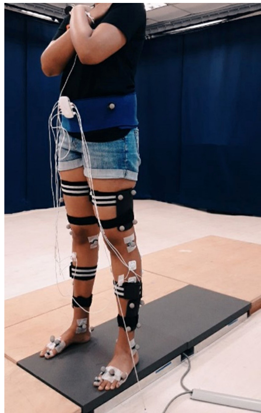
FIGURE 1 | Static trial for a subject with the placement of motion capture markers, Biosignalsplux SEMG electrodes and MART bands.
