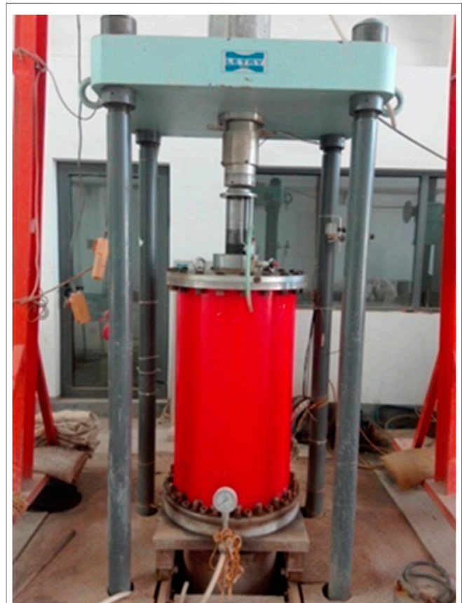
FIGURE 1 | Large-scale static triaxial apparatus.
