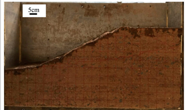
FIGURE 7 | Model of HRF embankment (after test).
