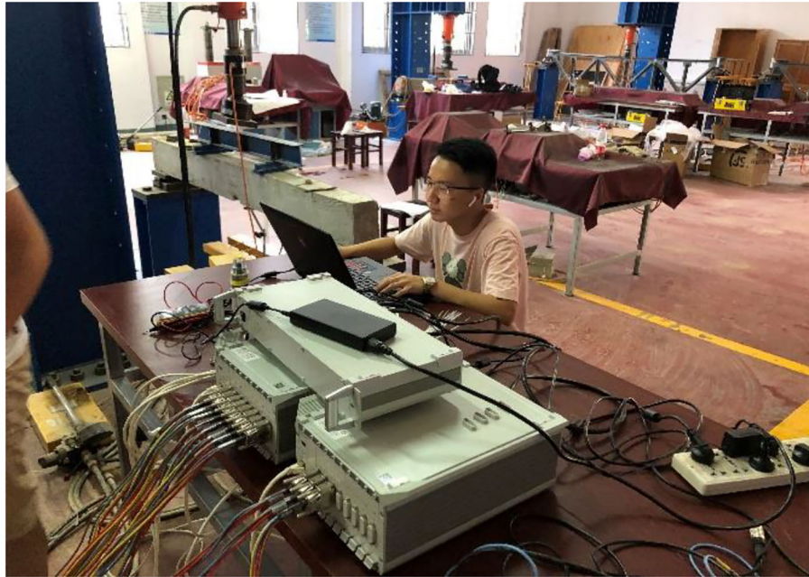
FIGURE 1 | Data acquisition system for shaking table test.
