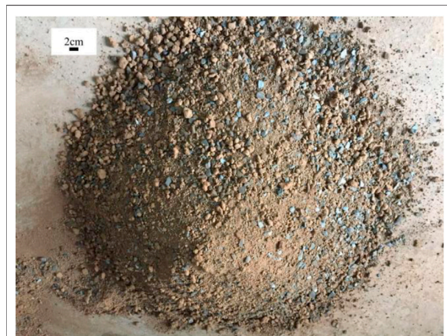
FIGURE 3 | Raw materials of rockfill embankment fillers.
