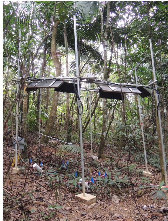
FIGURE 1 | Photograph of one of the experimental warming plots. Photo credit: Aura M. Alonso-Rodríguez.
