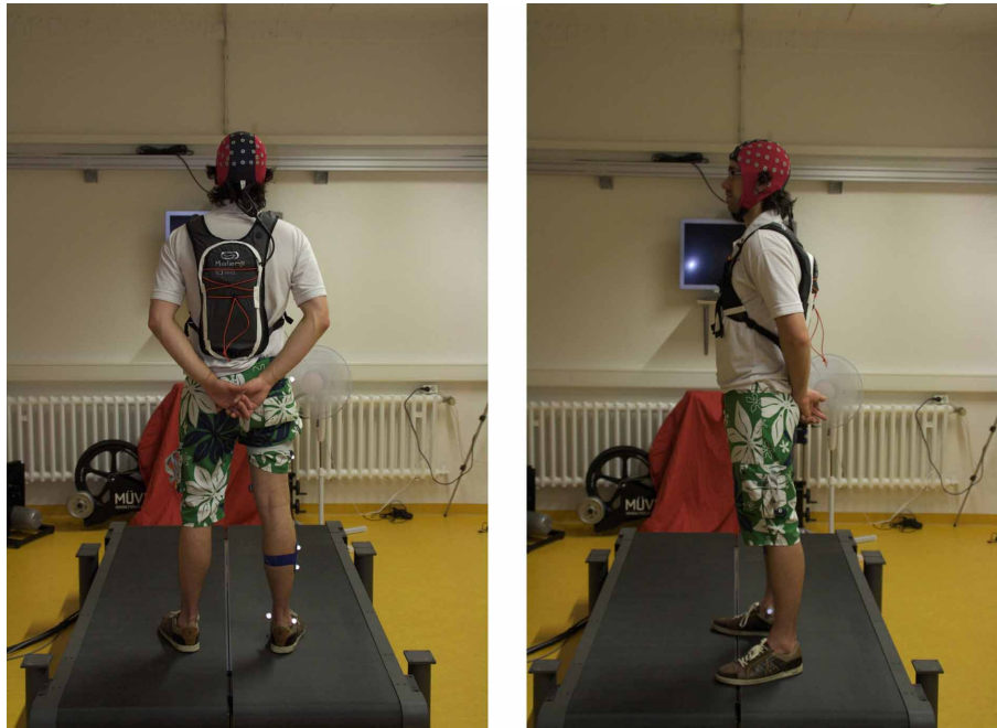
FIGURE 7 | ANT-Neuro eegosports™ wireless EEG system. Left: Posterior view: A study participant wearing the EEGSPORTS WaveGuard EEG cap. The cap cable goes inside the backpack where it connects to the amplifier and Ultrabook. Right: Lateral view.
