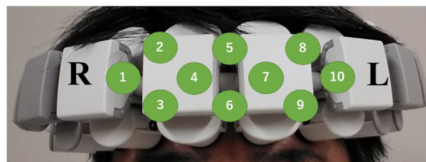
FIGURE 3 | Schematic of the probe unit, covering an area of 30 \times 105 \text{ mm}^2 on the participant's foreheads including both temples. This arrangement enabled the monitoring of cortical activation, mainly in the prefrontal cortex. All channels are labeled from 1 to 10.
