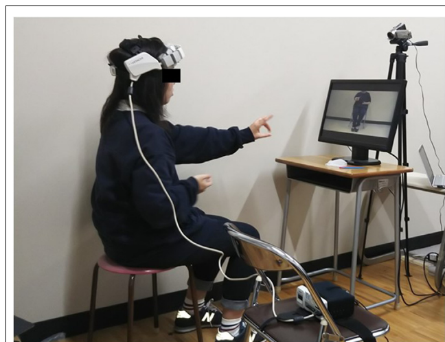
FIGURE 1 | Experimental setup of the antagonistic exercise tasks. The photograph shows a subject wearing a headset probe with the near-infrared spectroscopy (NIRS) device. The tasks being performed were recorded by the video camera. The participants had to imitate various tasks presented on a PC monitor placed in front of the subject at a viewing distance of 120 mm.
