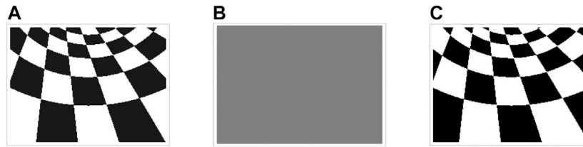
FIGURE 21 | (A) Black-and-white checkerboard visualizing the binary data stored in the locally distributed memristive memory bank previous to their retrieval. A white (black) pixel at row i and column j in this image reveals the on (off) resistance of the memristor in the M-CNN cell C(i, j) ( i \in \{1, \dots, M\}, j \in \{1, \dots, N\}, M = 177, N = 240 ). (B) Grey-scale image indicating the common -0.15 V-valued initial condition on each capacitor voltage. (C) Output binary image coding the steady-state output voltages of all the RECALL M-CNN processing elements. A black (white) pixel in correspondence to the i^{\text{th}} row and j^{\text{th}} column of this image denotes a positive (negative) saturation level +(-)v_{\text{sat}} for the steady-state output voltage of the cell located in the corresponding position of the memristive cellular array.
