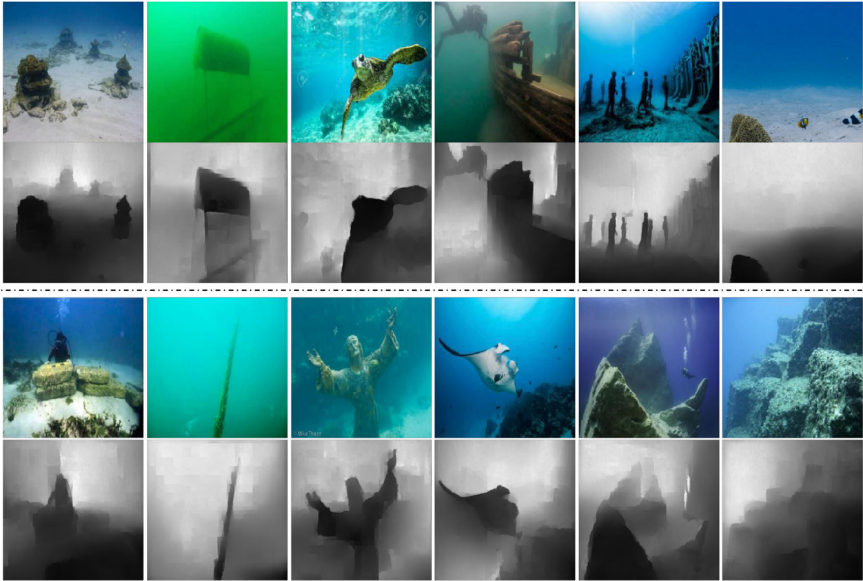
FIGURE 5 | The results of our model for depth map estimation. Every two rows from top to bottom are real underwater images with different illumination and scattering conditions and the results of our model for depth map estimation.
