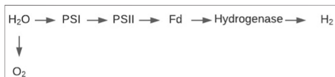
FIGURE 8 | Photosynthetic reaction scheme for bio-photolysis hydrogen production.
