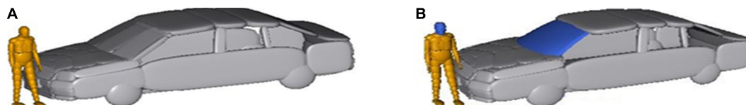
FIGURE 7 | (A) MB model of vehicle and VRU and (B) coupled vehicle and VRU model. MB, multibody; VRU, vulnerable road user.
