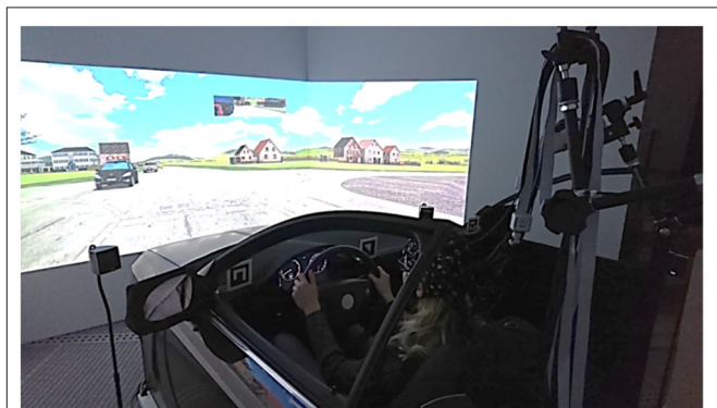
FIGURE 1 | Virtual reality lab driving simulator at OFFIS Institute of Information Technology, Oldenburg—photograph of experimental setup. The participant's brain activity is measured with whole-head fNIRS system while they are driving in the urban traffic.
