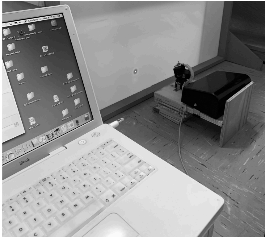
FIGURE 2 | A photograph of the set-up used to project moving laser spots on the wall or floor of the arena. Note the expanded diameter (5 mm) of the laser spot due to scatter by the translucent screen upon which it is projected.
