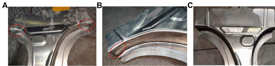
FIGURE 5 | Formed parts: (A) Part No. 1, with full BHF; (B) Part No. 2, with half BHF; (C) Part No. 3, no BHF.
