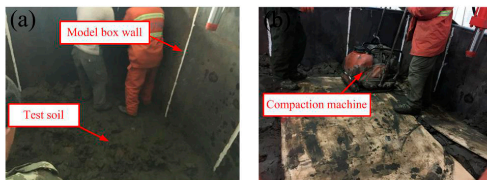
FIGURE 4 | The process of soil preparation: (A) Soil filling, (B) Soil compaction.
