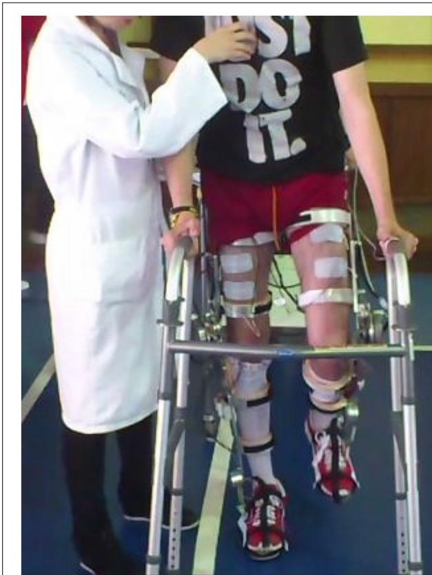
FIGURE 2 | Experimental setup for data collection and testing hybrid gait training with Kinesis overground robot.
