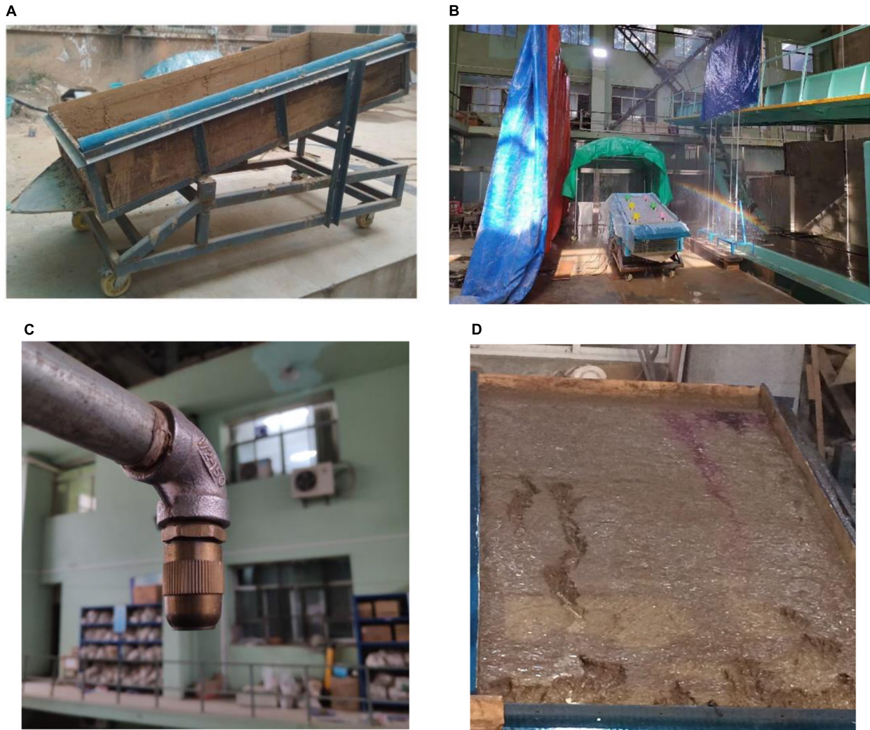
FIGURE 1 | The experimental soil flume (A), calibration rainfall intensity (B), rainfall simulator (C) and runoff over the flume (D).
