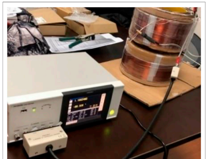
FIGURE 12 | Winding AC equivalent resistance experiment.
