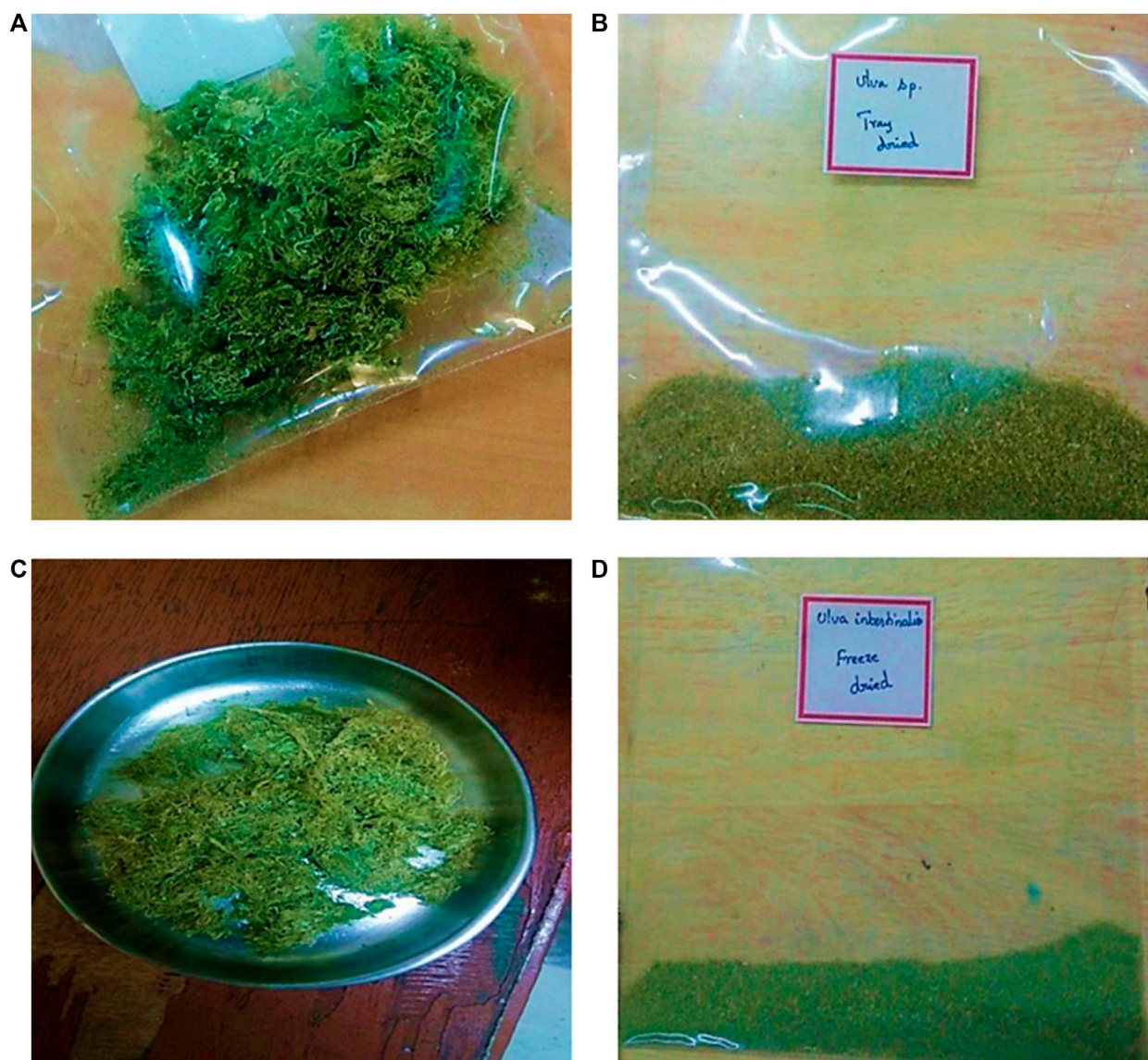
FIGURE 1 | Samples of U. intestinalis used for Soxhlet extraction using ethanol. (A) Tray-dried sample (B) powdered form of tray-dried sample. (C) Freeze-dried sample (D) powdered form of freeze-dried sample.
