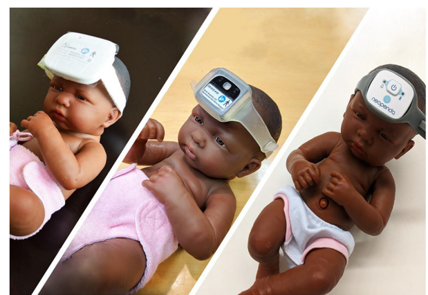
FIGURE 2 | Prototypes of neoGuard hardware versions v1.0 (left), v2.2 (center), and v3.0 (right).
