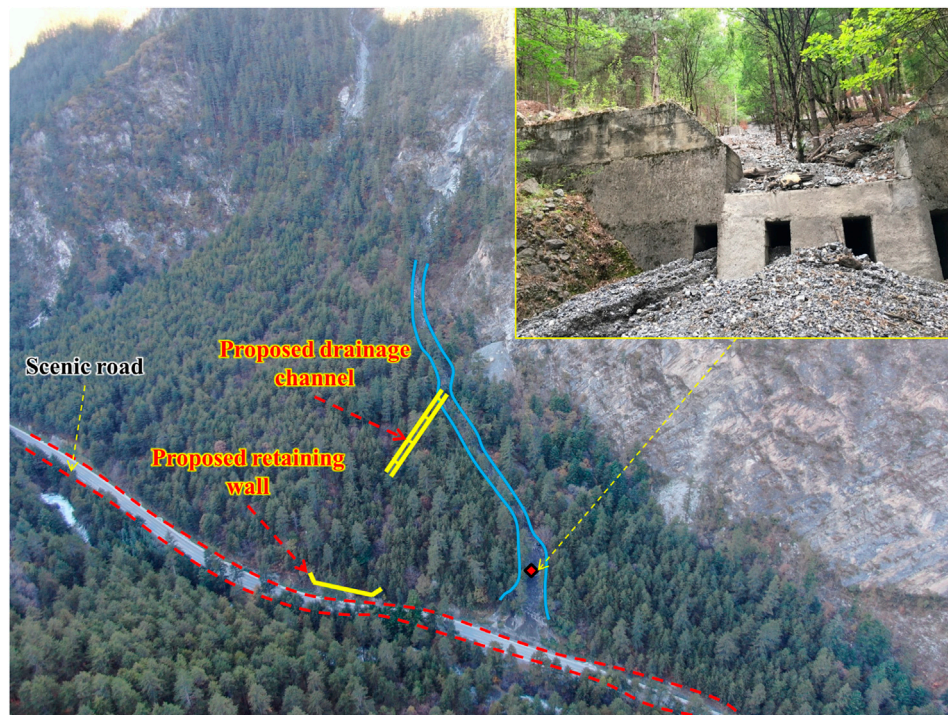
FIGURE 6 | Control engineering layout of Pingshitou Gully (after the debris flow event on July 22, 2019). The blue line in the figure represents the main channel. The drainage channel and the retaining wall in the figure are the proposed engineering projects described in Application of the Planning Method for the Xiajijie Lake, Zhuozhui, Pingshitou, Xuan, and West-Zhuozhui Debris Flow Gullies section.
