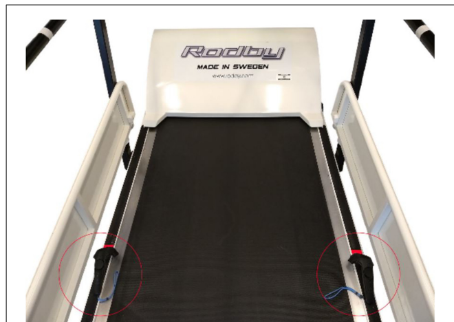
FIGURE 4 | During calibration process, the hand controllers are physically placed on the treadmill as illustrated.
