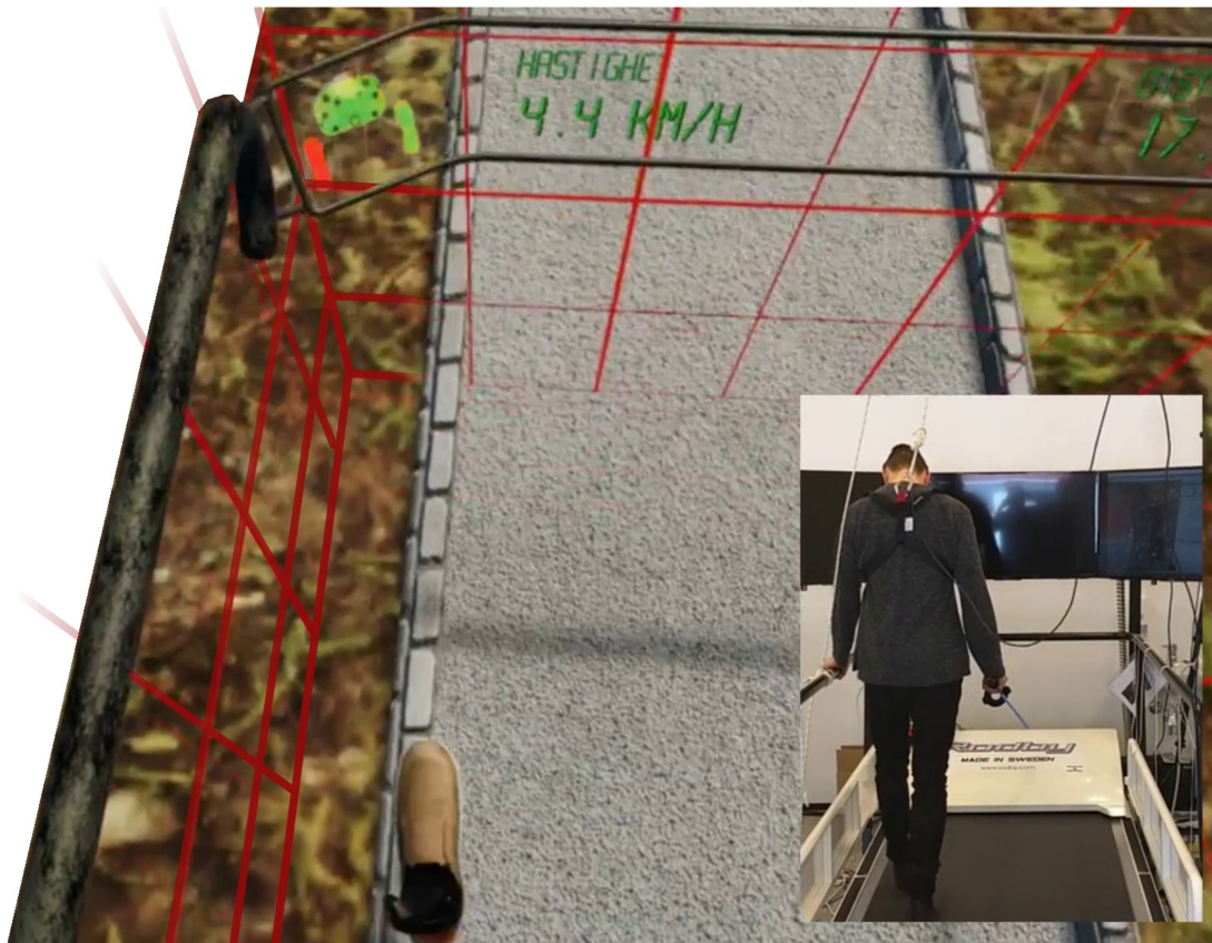
FIGURE 2 | When the player steps toward the limits of the game area, a grid is visualized. If the player steps past the game area, the grid turns red and the treadmill stops automatically. External safety measures such as harness and treadmill railing is recommended.
