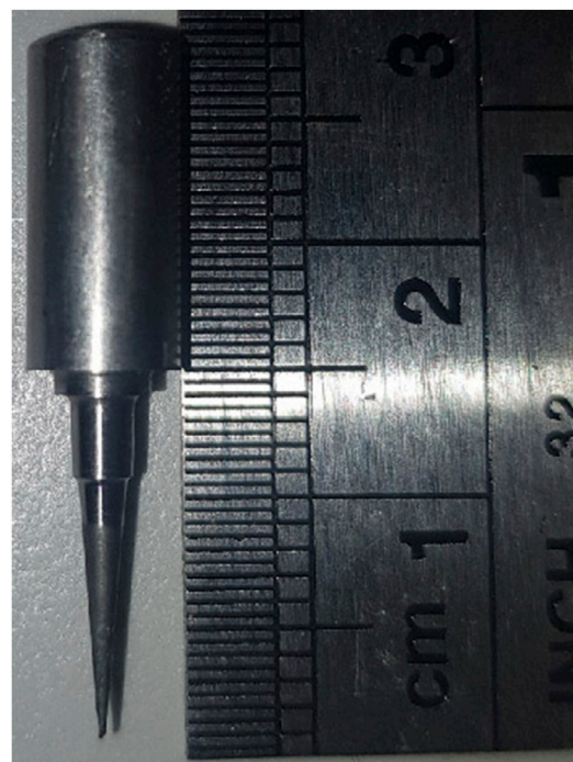
FIGURE 4 | Conical indentation tip with an internal angle of 9.5^\circ and a tip radius of 250 \mu\text{m} .
