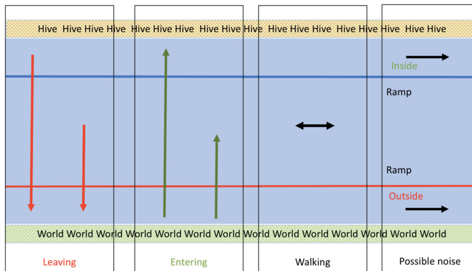
FIGURE 5 | Event classification policy based on trajectory endpoints. The entrance to the hive is at the top and the outside world is at the bottom. Red arrows represent exit events (leaving): these trajectories start inside the ramp and end below the threshold represented by the red line. Green lines represent entrances: these trajectories start at the bottom and end inside the ramp. Black lines represent ignored trajectories that are the result of tracking interruptions or of bees that dwell in a single area but never enter nor exit.
