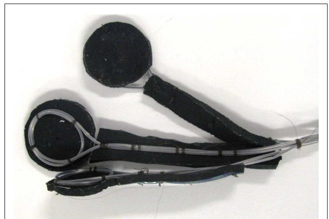
FIGURE 9 | Photograph of completed carbon fiber movement detection loops.
