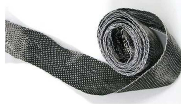
FIGURE 1 | Roll of carbon fiber tape from which bundles of “wire” can be extracted.
