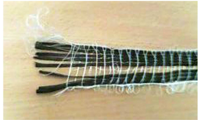
FIGURE 4 | Extracting carbon fiber bundles from woven tape.
