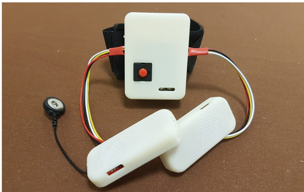
FIGURE 2 | The figure shows the sEMG bracelet, developed to reduced the disturbances coming from the sensor wires, with its central unit and the other two smaller ones containing the sEMG sensors.
