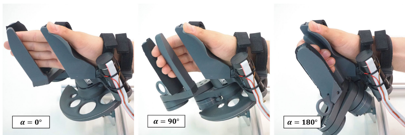
FIGURE 11 | Hand movement sequence from full finger extension to 180° flexion for a hand of size medium-large .
