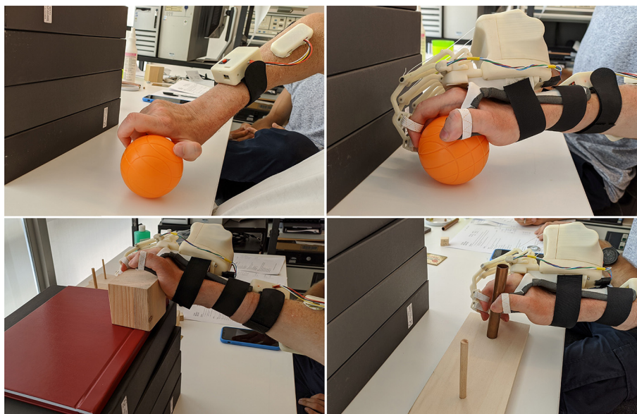
FIGURE 7 | The figure shows some pictures taken during the test: (i) on the top-left, the cricket ball grasping (G5) performed without the HES, (ii) on the top-right, the same task performed with the HES, (iii) on the bottom-left, the wooden block grasping (G1) is shown, while (iv) on the bottom-right, the alloy tube gripping (GR2) is visible.
