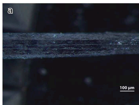
FIGURE 6 | Electrical conductivity of alginate-graphene fibers. (a) Light microscope image of the fiber used as the working electrode. (b) Cyclic voltammograms of alginate-graphene fibers. Potential was scanned between -0.5 and +0.8\text{ V} (vs. Ag/AgCl) in simulated body fluid (SBF) at 100\text{ mV/s} .
