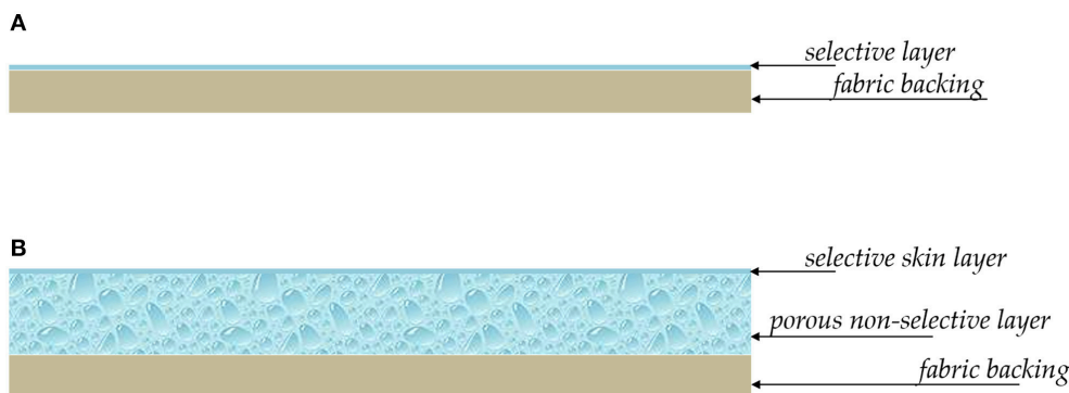
FIGURE 7 | Structure of composite (A) and asymmetric (B) membranes for OSN.
