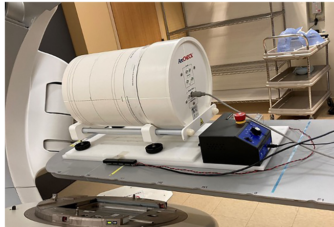
FIGURE 3 ArcCHECK detector placed array on the motion platform before dose measurement.
