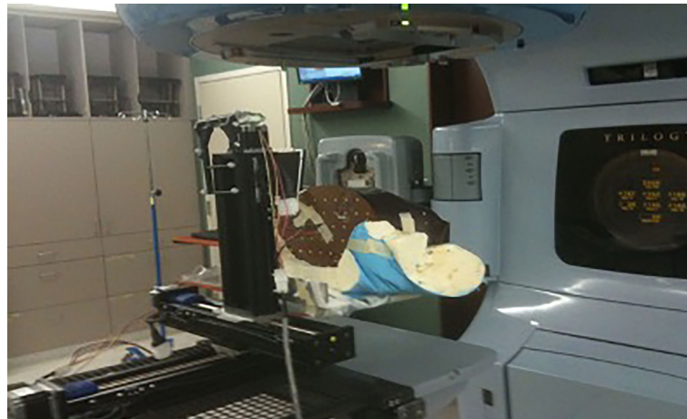
FIGURE 1 Experimental setup showing the RANDO phantom immobilized with alpha-cradle on a motion platform.
