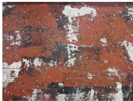
FIGURE 10 | The impact of underwater cleaning using a handheld polypropylene or wire brush.
