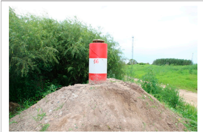
FIGURE 3 | Marker-stake for surface displacement measurement.
