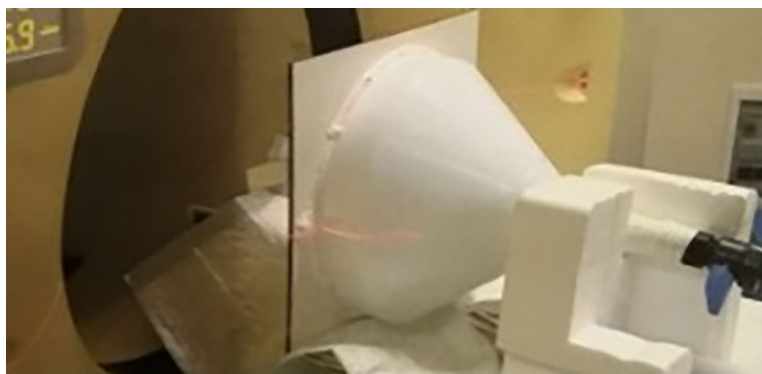
FIGURE 4 Our funnel phantom (plastic filled with water).
