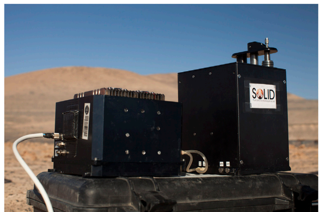
FIGURE 5 | SOLID, the Signs of Life Detector, developed at the Centro de Astrobiología (Center of Astrobiology) in Spain. Photo credit: Víctor Robles.
