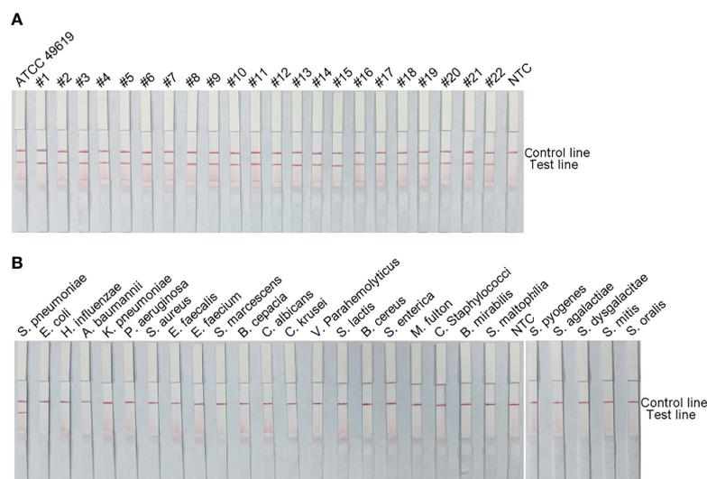
**FIGURE 4** | The RPA-LFS assay's specificity. *S. pneumoniae* clinical isolates **(A)** and other common pathogens **(B)** were tested. The positive control was *S. pneumoniae* (ATCC 49619). Each bacterium's species name is shown at the top of each strip. The NTC strip is a no-template control. The reactions were carried out for 30 minutes at 37°C.
