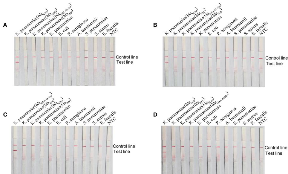
**FIGURE 4** | Specificity of the RPA-LFS reaction system. The name of the template added to each reaction is labeled above the corresponding band. Primer-probe combinations of *bla*<sub>KPC</sub> **(A)**, *bla*<sub>NDM</sub> **(B)**, *bla*<sub>OXA-48-like</sub> **(C)** and *bla*<sub>IMP</sub> **(D)** were added to the reactions. The NTC strip was used as a control reaction without a template.
