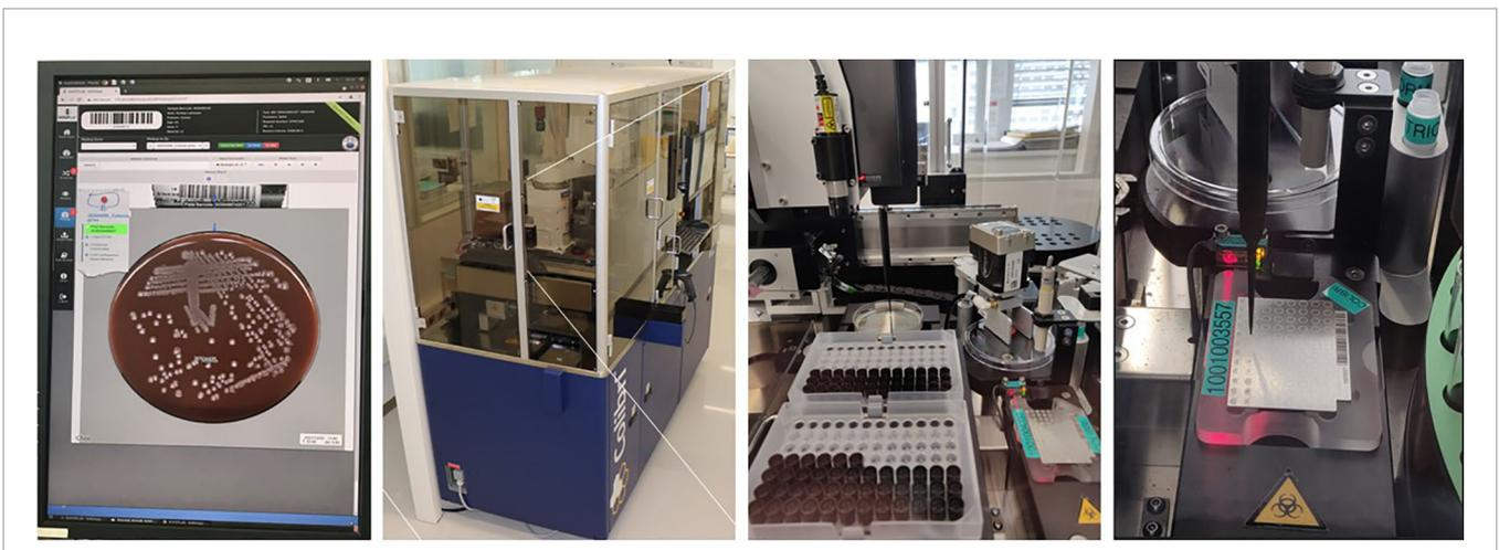
**FIGURE 3 |** Automated System for Colony Picking and MALDI-TOF Targets Preparation (Copan Colibri™). A pipetting system permits: i) the picking of the specific colonies determined by the technologists during the reading step on the WASPLab screen; ii) the transfer of the microorganisms’ cells on the MALDI-target; and iii) the deposition of the matrix. Two protocols are available with (or without) extraction using a formic acid. Source of all images: A. Cherkaoui, Geneva University Hospitals.
