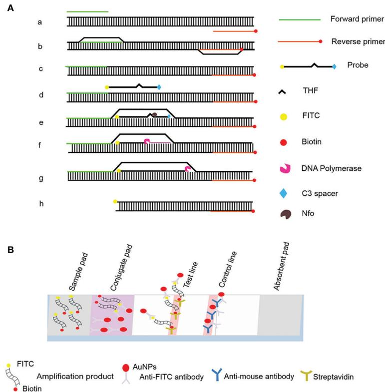
**FIGURE 1** | Schematic diagram of the RPA-LFS method. **(A)** Principle of RPA amplification. DNA strands are represented as horizontal lines, and base pairing is represented as short vertical lines between DNA strands. Base pairing is indicated as a short vertical line between DNA strands. **(B)** Schematic representation of the lateral flow strip (LFS) working principle. The shapes and their representative molecules are listed below the graphic.
