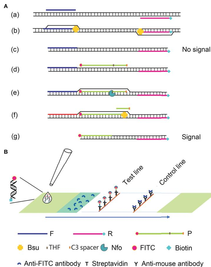
**FIGURE 1** | Schematic diagram of the RPA-LFS method. **(A)** The RPA amplification principle. Base pairing is represented as short vertical lines between DNA strands, and DNA strands are represented as horizontal lines. Base pairing is represented by a short vertical line connecting two DNA strands. **(B)** A schematic representation of the lateral flow strip (LFS) operation. The shapes and the molecules that represent them are listed below the graphic.
