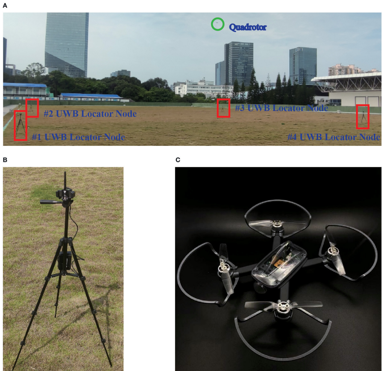
FIGURE 5 | The experimental preparations for online path planning and tracking. (A) The experimental site for online path planning and tracking of multi-UAVs. (B) The UWB locator node. (C) A micro quadrotor with UWB tag.
