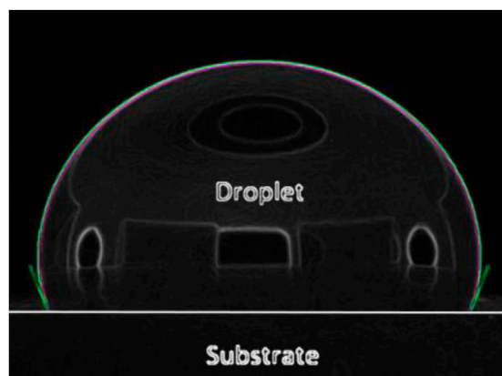
FIGURE 2 | Contour fitting—green line—of liquid steel sessile droplet.
