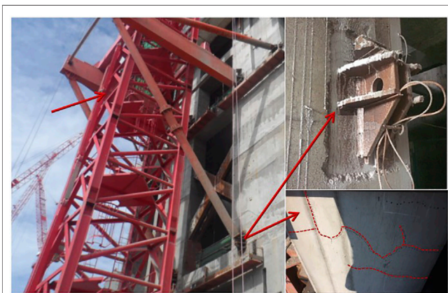
FIGURE 2 | BFJ of tower crane and cracks.
