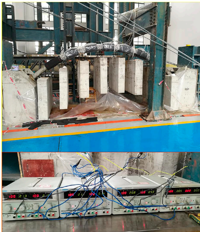
FIGURE 5 | Actual corrosion process of the arch model.
