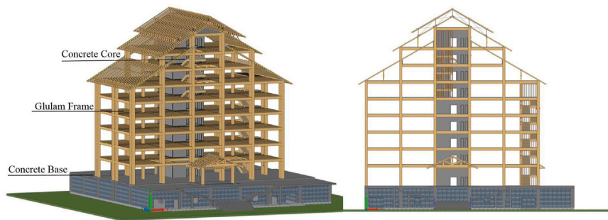
FIGURE 1 | Sketch of 10 storey timber-concrete hybrid building.
