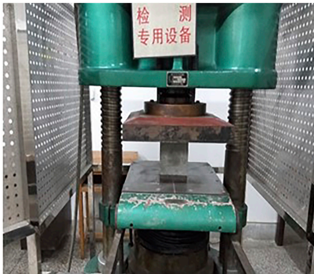
FIGURE 7 | Concrete performance test device.
