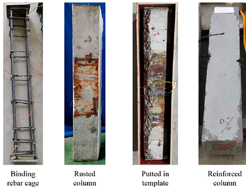
FIGURE 2 | Main process of specimen fabrication.
