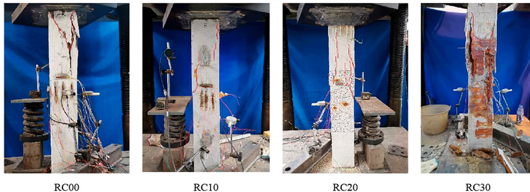
FIGURE 5 | Failure mode of the unreinforced specimen.
