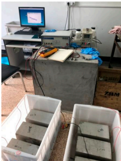
FIGURE 5 | Accelerated corrosion method and measurement of electric polarization parameter.
