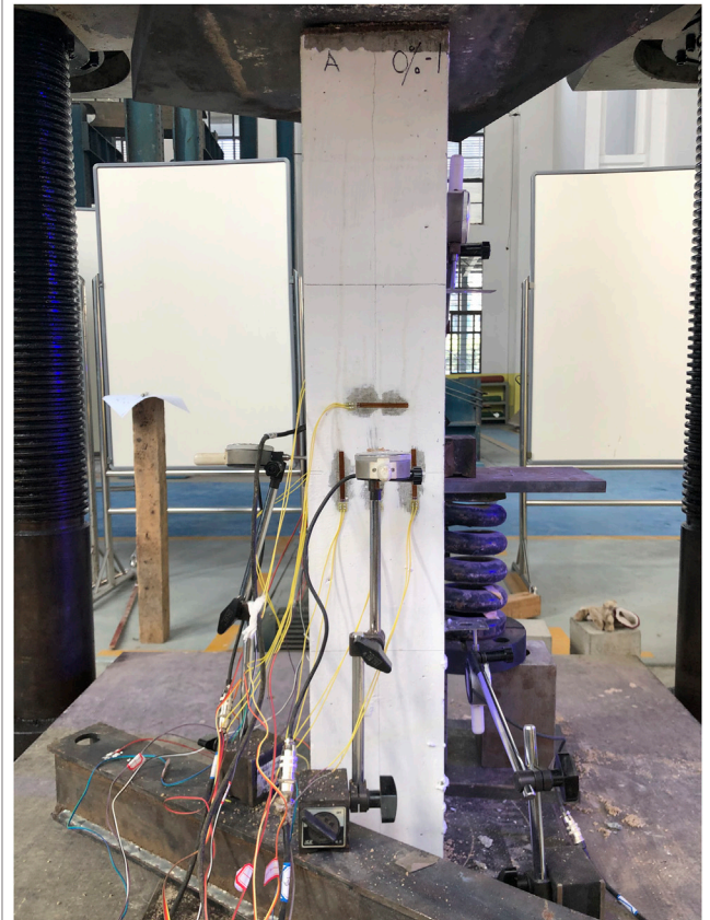
FIGURE 4 | Loading set-up of the axial compression test.
